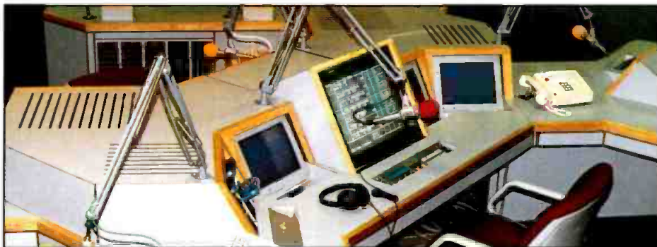
A touchscreen system controls the on-air operation for WCCO-AM's talk-radio format in Minneapolis.
